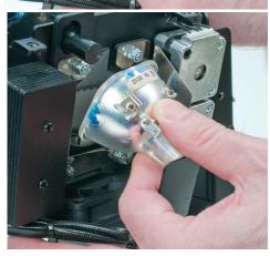
Carefully disconnect the two wires that are connected to the lamp's reflector. Firmly grab the moving head to hold it in place. Gently press the lamp down, and gently pull the top of the lamp out of the lamp holder. *Note:* Never touch the lamp located within the reflector with your bare hands.
