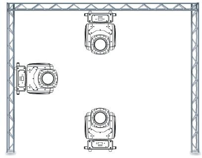
The Vizi Beam RXONE is fully operational in three different mounting positions, hanging upside-down from a ceiling, sideways on trussing, or set on a flat level surface. Be sure this fixture is kept at least 12m (40ft) away from any flammable materials (decoration etc.). Always use and install the supplied safety cable as a safety measure to prevent accidental damage and/or injury in the event the clamp fails (see next page). Never use the carrying handles for secondary attachment.
