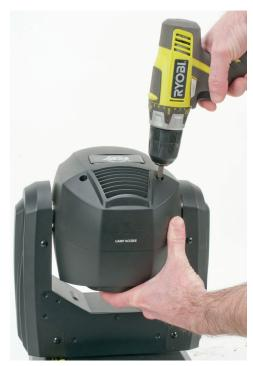
Replacing the lamp is relatively easy. Unplug the unit from its power source. Allow the unit 15 minutes to cool down. Remove the shell that says "Lamp Access" on the rear. Start by unscrewing the four phillips screws that hold the shell in place. Once the screws are unscrewed remove the shell. You will now have access to the lamp.
