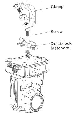
Screw one clamp via a M12 screw and nut onto the Omega holders. Insert the quick-lock fasteners of the first Omega holder into the respective holes on the bottom of the Vizi Beam RXONE. Tighten the quick-lock fasteners fully clockwise. Pull the safety-cable through the openings located on the base plate and over the trussing system or a safe fixation spot. Insert the end in the carabine and tighten the safety screw.
