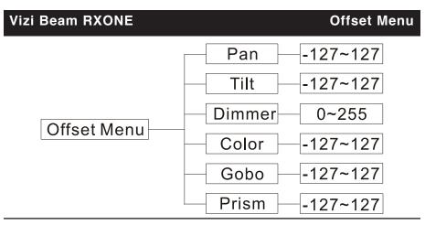
To enter the Offset Menu, press the ENTER button for at least 5 seconds. In this submenu you are able to adjust the home position of the pan, tilt, shutter, color wheel, gobo, and prism.
